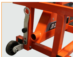
DUST EXTRACTION PORT Ø 40mm
