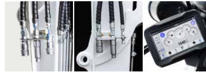
1st AUX hydraulic on arm 2nd AUX hydraulics with drain line 7-inch display
