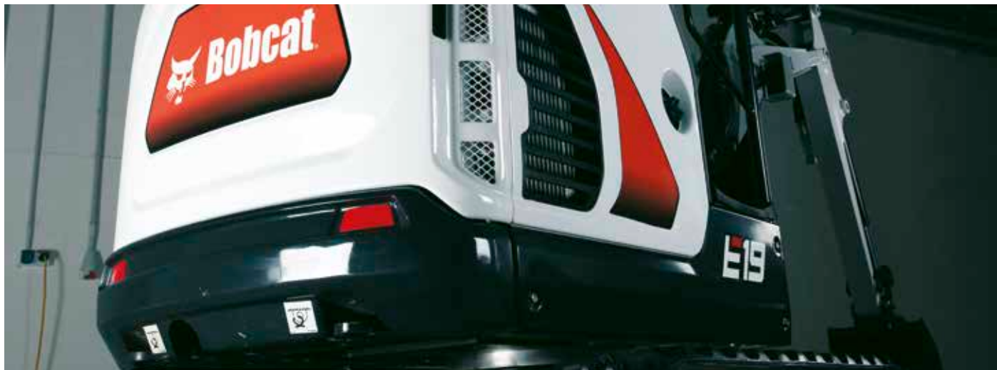
Casted counterweight protects the tailgate
