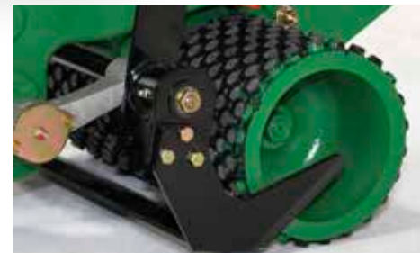
KNOBBY TREAD DRIVE TIRES MOLDED TO HUB
