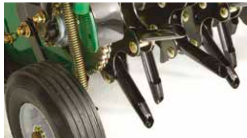
STANDARD 0.75" (19 MM), HARDENED ALLOY STEEL CORING TINES
