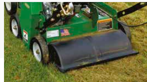
BUBBLE SHIELD PREVENTS THATCH BUILDUP
