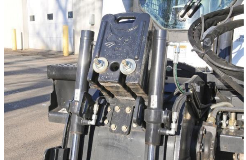
Brackets and hardware hold the weights securely to the 18-inch and 24-inch planers
