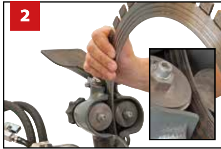
Place the blade between the rollers. Make sure the guide roller is placed correctly into the grooves of the blade.
