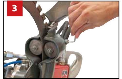
Gently (NOT tightly) adjust the support roller against the blade using the hex key. NB: The roller adjustment is eccentric - if you tighten too far to the right it will become loose again.
