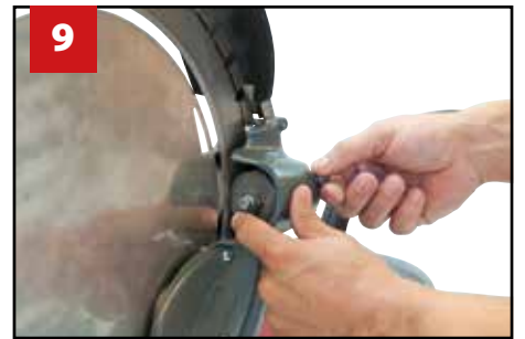
If the support roller is correctly adjusted you can turn the roller by the finger. If it cannot turn it is too tight.
