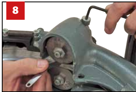
Re-adjust the support rollers > loosen the screw counterclockwise with the hex key, use the feeler gauge to adjust the gap between the support roller and the blade > turn the screw clockwise until the gap matches the feeler gauge.
