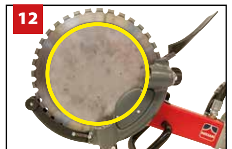
Check that the distance between water blade and blade is the same full circle.
