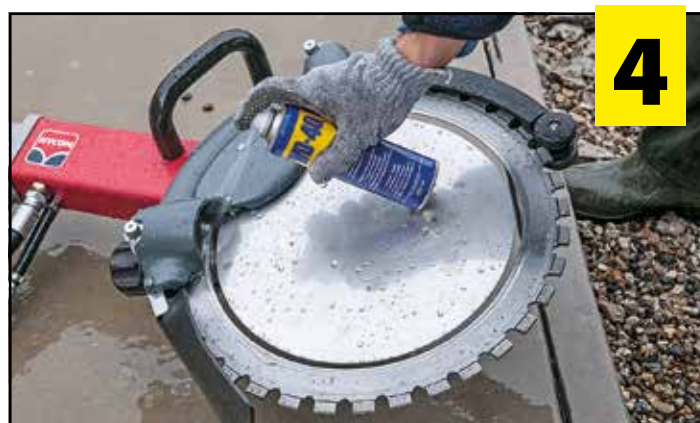
Finally spray all parts with WD-40 or equivalent water-displacing spray
