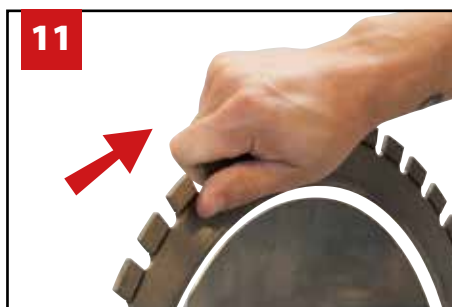
You must be able to turn the blade by the hand.
