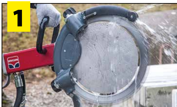
Let the ring blade spin free for minimum 30 seconds after EACH JOB. Clean water will flush the rollers.
