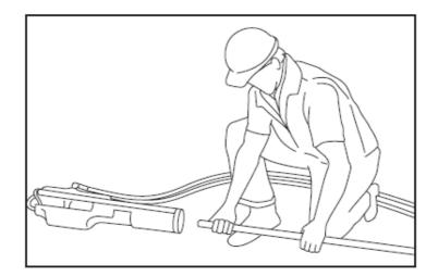
• Lift the post and driver to a vertical position as shown in fig. 2
