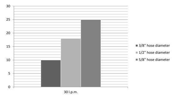
Pressure from power pack: 150 bar., Flow: 30 l.p.m., zero elevation, 2 set couplings per 10 m hose.
