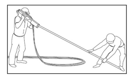
• To start the post driver move the control valve to the ON-position. Fig 3
